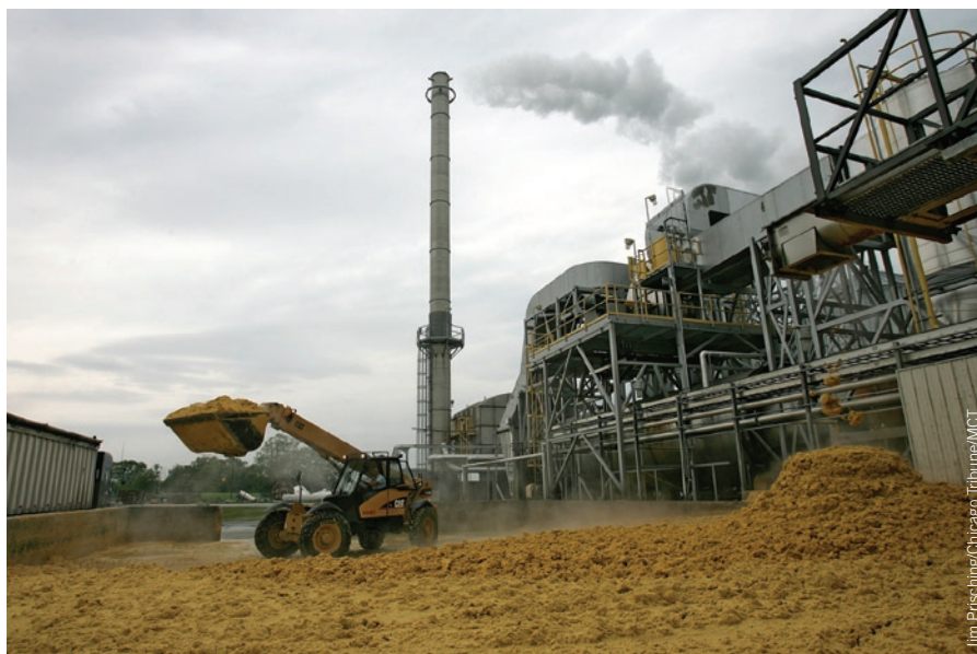
Leftover corn product after distilling at the Adkins Energy Ethanol Plant in Lena, Illinois. Second-generation biofuels that use alternative feedstocks are expected to replace corn-based ethanol.
